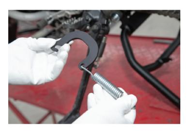
10. Attach the hook onto the mounting rod as shown in the photo.
