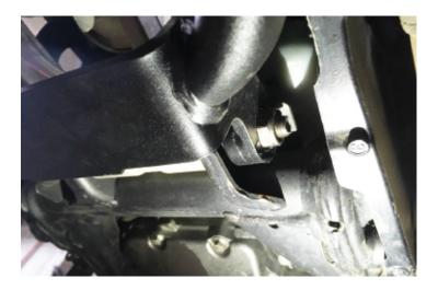
4. Once the right side tab has been mounted, proceed to lining up the left side tab with the corresponding mounting hole.
