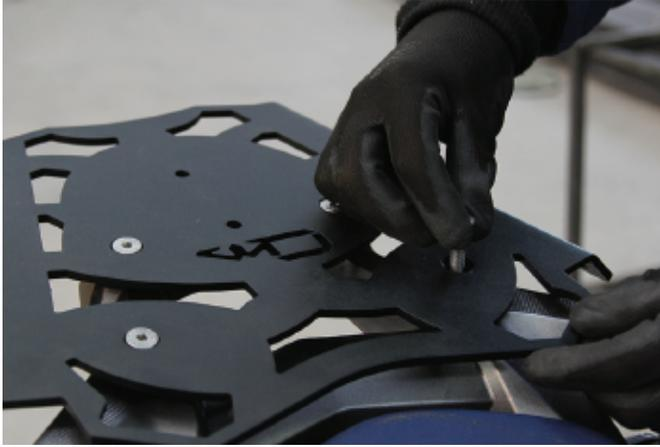
4. Insert the washers and thread on the nyloc nuts.
