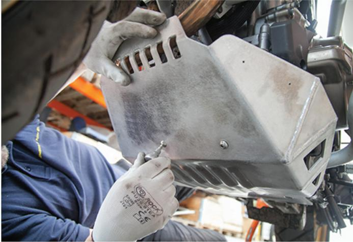
8. Insert and hand-thread the M8x12 mm Allen bolts after lining up the rear mounting holes.
