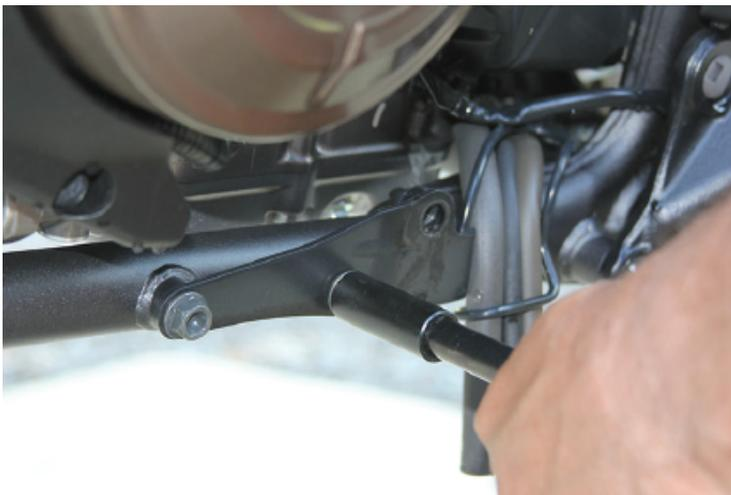
2. Take the supplied skid plate mount cross brace and place it on the frame underneath the engine.
