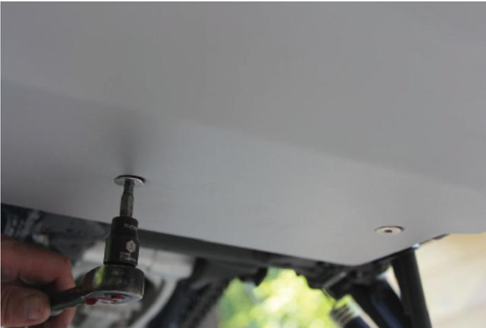
6. Tighten the skid plate mount bracket bolt now using a 12mm socket and ratchet. Factory recommended torque specs 44Nm.
