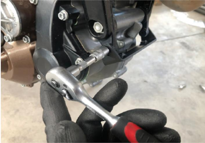
4. Make sure the bracket is loose enough to line up the mounting holes on the bracket and the skid plate.
