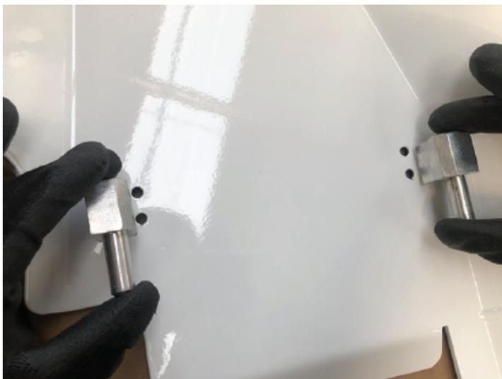
6. Hand thread the supplied M6 Allen bolts through the bottom.
