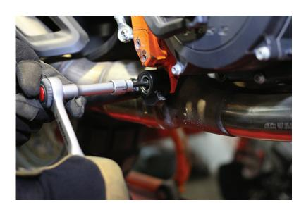
10. Fully tighten all the bolts, double-check that the hooks have properly engaged (sittingin the notching).
