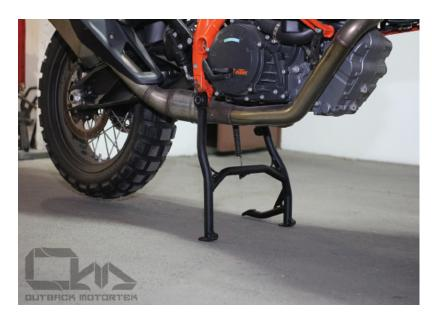
You've completed installing the centre stand. Please test the product's functionality numerous times by lifting the bike and taking it off the centre stand.
