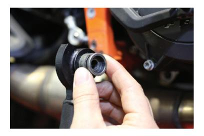
4. Mount the centre stand and thread in the M8x35 Hex/Torx bolts on both sides. Use thread locking fluid.
