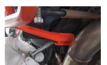
12. Mount the right side front skid plate mount (short piece). Replace the factory engine mount bolt. Leave it loose for now.
