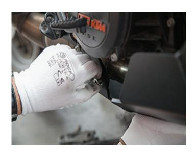
18. Finally, go ahead and tighten all the bolts and nuts to torque specs and make sure to check again after going out for a test ride.
