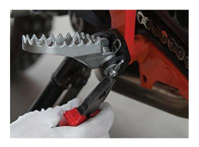
2. **Highly recommended that you wear safety glasses!** Next, you'll have to remove the Clevis pin. Be very careful, torsion spring may come flying at you, so make sure to place one hand over the foot peg bracket.
