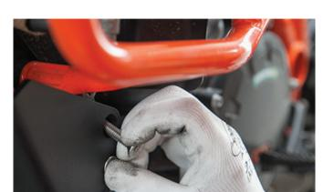
16. Insert the 8mm diameter Allen bolts through the left side rear mount. Thread the supplied nyloc nuts on the end. Leave it loose.
