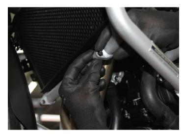
18. Tighen all four bolts to the recommended torque specs.
